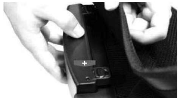
Fig. 31: Insert the battery
