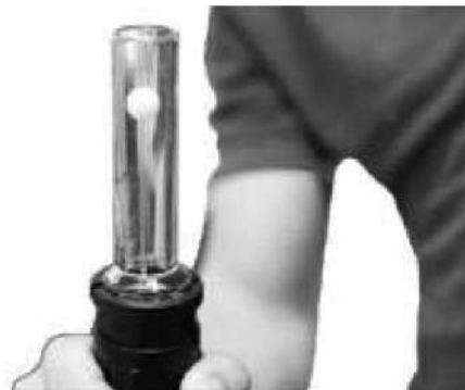
Fig. 17: Vertical position of the flow meter
