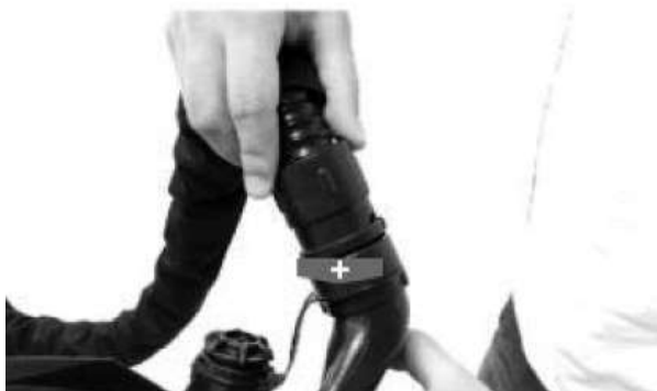
Fig. 19: Dismantling the hose on the helmet side
